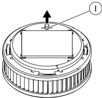
Fig. 20 Pulling out the activation button
